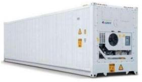
Temperature control scope : 0 ± 10°c Default temperature set at 0°c
